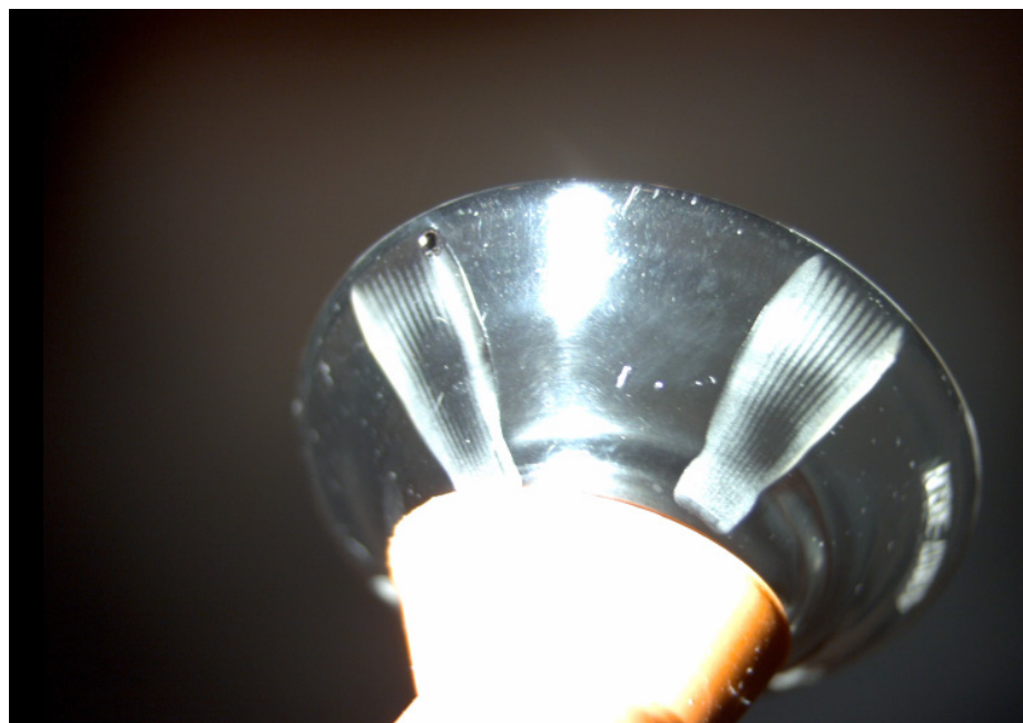
Figure 6: Back-surface channels added to a 19.5mm, quadrant-specific lens, to reduce suction.
