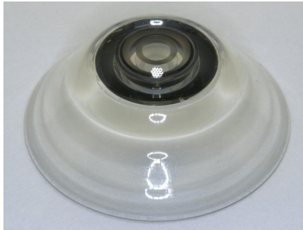
Figure 3. Scleral lens-based telescope. Image courtesy of Glenn Schuster.
