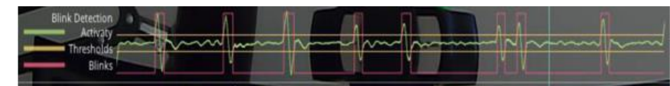
Figure 3. Wearable eye-tracking headset player timeline example of blink rate and interblink interval detection for a 13-second recording of the right eye only, showing 8 blinks (plotted in green, with pink line above and below), interval between blinks (plotted as pink straight line below; bottom). The post-hoc predetermined blink detection onset and offset thresholds are shown in yellow lines (middle)
